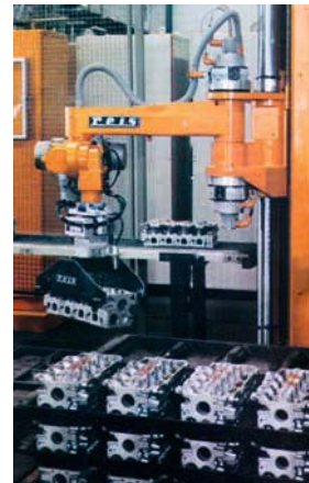
ROBOT 625 handling motor blocks (source: Fraunhofer IPA)
