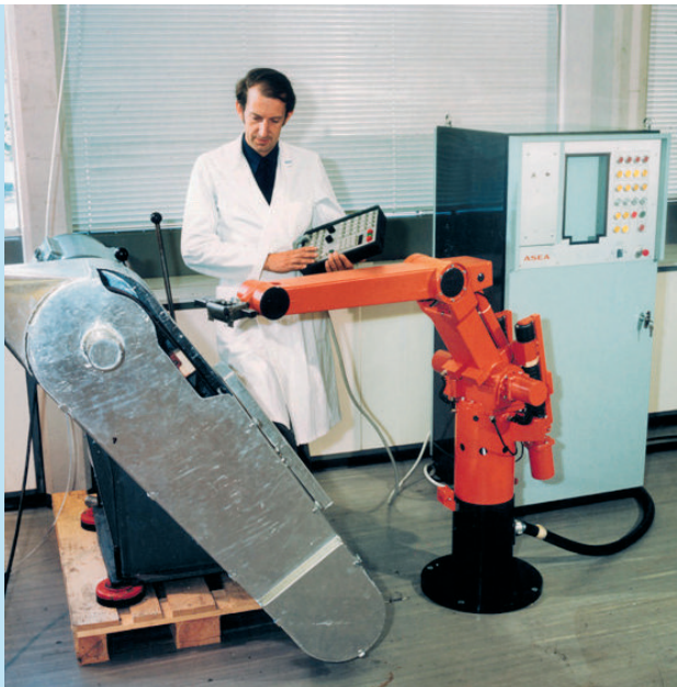
IRB 6 by ASEA with 6kg payload capacity (source: ABB)
