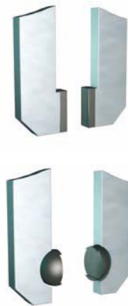
A simple method to ensure plane surface contact
