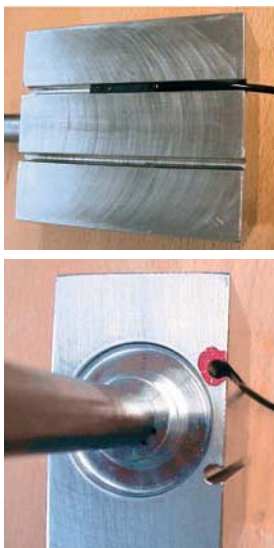
measuring the piston position by magnetic sensors in the tongue
