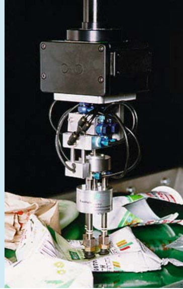
Grippers for foreign or hazardous materials can deform workpieces
