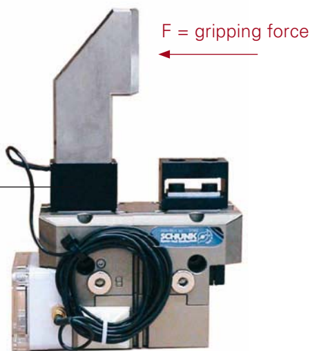
DMS strain gauge bridge as measuring adapter
