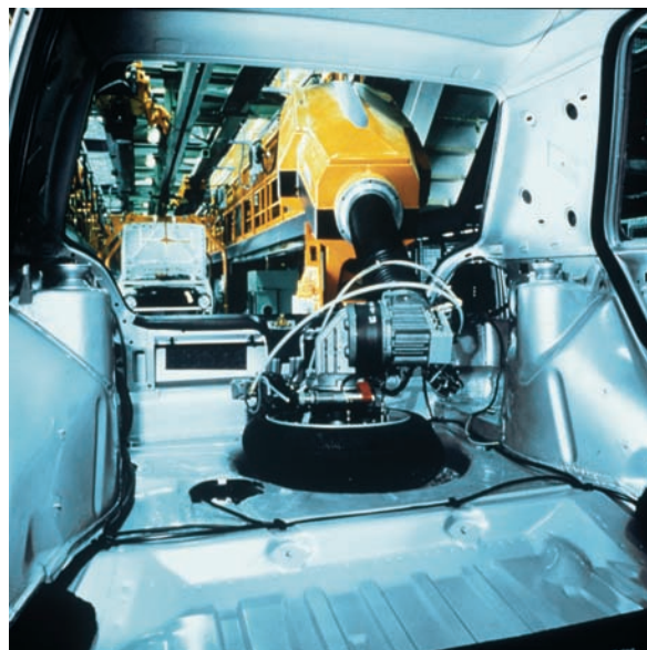
Typical application of a VW robot for inserting the spare wheel into the Golf II (source: Fraunhofer IPA)
