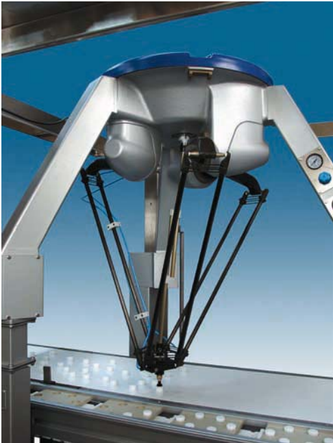
Parallel kinematics mounted to the ceiling by a specially designed frame (source: SIG Packsystems))
